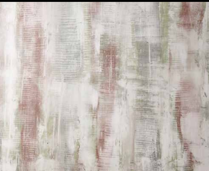
STUCCORINO + Pigment 2805 + Goldglimmer mittel STUCCORINO + Pigment 2906 + Goldglimmer mittel STUCCORINO + Pigment 2406 + Goldglimmer mittel + STUCCORINO Fresco Natur
